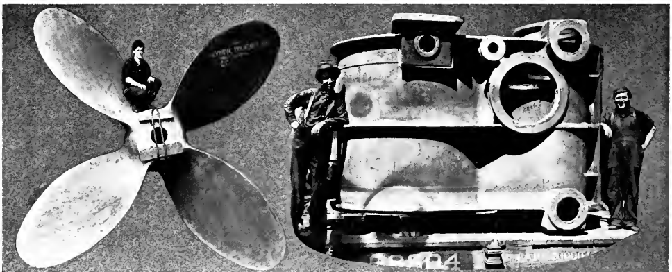
A large four-bladed propeller and a low-pressure cylinder cast at the plant of the Olympic Foundry Company, Seattle, Washington. This concern is turning out a great amount of heavy marine castings.
